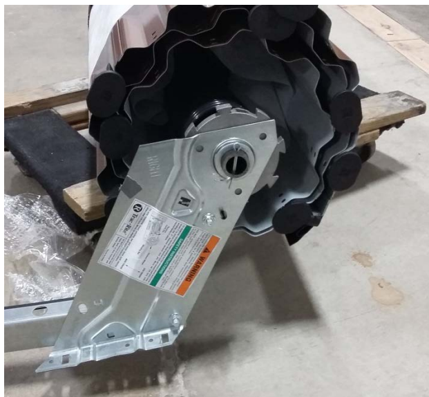
Photo No. 2 Door Brackets/Spring Assembly
